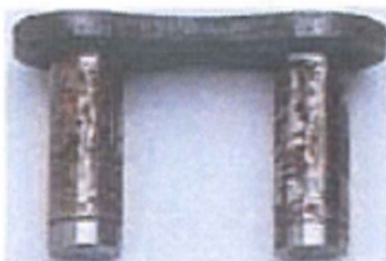
Wear caused by insufficient lubrication
